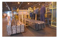
Floors can be made of hot rolled steel sections welded together, or constituted of galvanised cold formed joists and beams bolted together. In both cases, the cutting pattern of the structural components from standard lengths is carefully planned to reduce, if not eliminate, wasted materials. However, the steel off-cuts are collected in designated skips and sent to the suppliers for recycling.
