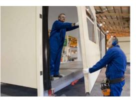
The wall panels are manufactured to be of the length of the wall in order to avoid redundancy in the structure, thus limiting the use of materials and resources. Furthermore, Yorkon has recently introduced a lower density material for insulation (40 kg/m<sup>3</sup> instead of 45kg/m<sup>3</sup>). This change in insulation specification, whilst having limited impacts on the thermal performance of the panels, has reduced the quantity of insulation materials used per unit built.
